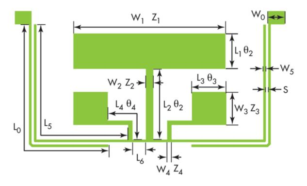
Each MMR is constructed of three stepped-impedance stubs (SISs) loaded symmetrically on a resonator with uniform impedance. By using such SISs, a bandpass filter with 48% fractional bandwidth was designed and fabricated. It features as much as 50-dB upper stopband rejection with 35-dB lower stopband rejection.
